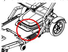
2) Fold the seat backrest down and then fold the tiller downward
