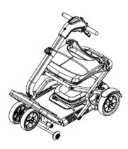
3) Lock the scooter onto the open position by pulling the seat up and pushing the tiller forward until a click sound is heard.
