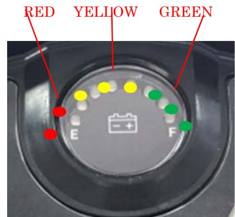
The remaining power suggested by the battery indicator will vary by the actual driving time incurred and how you drive. Repeated starting, stopping, climbing will consume the power more quickly.
