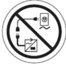
**PROHIBITED!** Never use an extension cord to plug in your battery charger. Plug the charger directly into a properly wired standard electrical outlet.
