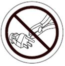
**PROHIBITED!** Removal of grounding prong can create electrical hazard. If necessary, properly install an approved 3-pronged adapter to an electrical outlet having 2-pronged plug access.
