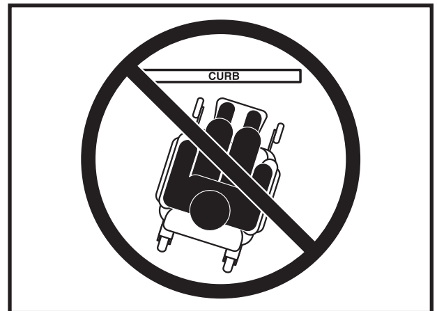
Figure 5. Incorrect Curb Approach
