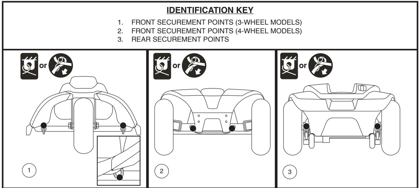
Figure 9. Securement Points (Identified with black dots)
