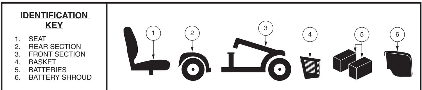
Figure 27. Disassembled Scooter
