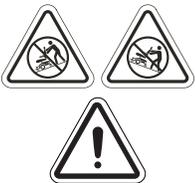
**WARNING!** Do not use the scooter while the drive motors are disengaged! Do not disengage the drive motors when the scooter is on an incline or decline, as the unit could roll on its own! Only engage the freewheel mode when on a level surface.
